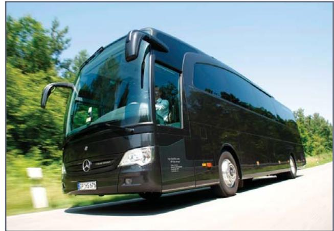
*“We originally had Mirror Polished wheels, which required a lot of maintenance to keep them shiny. We started retrofitting the vehicles with Alcoa Dura-Bright® wheels in 2009, as these wheels can be cleaned very quickly and easily. All our coaches are cleaned on a daily basis, which is a normal procedure for VIP vehicles,” explains Holger Schnizler. “Customers expect our VIP coaches to have a perfect appearance, and with Alcoa Dura-Bright® wheels, that is exactly what they get.”*
